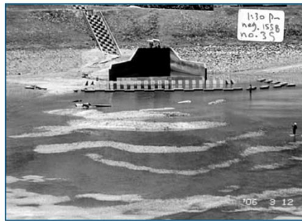
Fig. 1. Erosion from a hydropower tunnel
